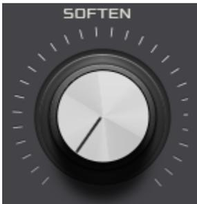
Adjusts the softness of KClip's oversampled clipper process. This control is active in all Soft Modes other than Crisp, which has a fixed soft curvature.
