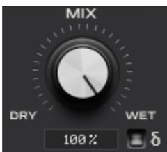
The Mix control adjusts the final ratio of wet (processed) to dry (unprocessed) signal. The Delta function toggle (δ), when enabled, allows you to listen to only the changed audio signal, irrespective of the value set on the Mix control.
