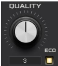
Adjusts the number of times oversampling used for realtime monitoring, in powers of two (2x, 4x, 8x, 16x, and 32x oversampling from 1-5.) Higher values equal better sound quality, at the expense of CPU. The "Eco" toggle enables a low latency oversampling filter topography, useful for tracking in realtime and on slower CPUs.
