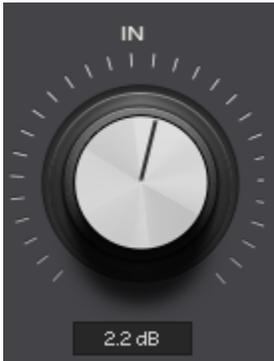
Adjusts the amount of gain boost (or reduction) to be applied to the incoming signal prior to oversampled clipping.
