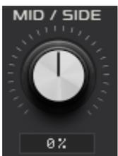
Adjusts the mid/side stereo field ratio. When centered, the input stereo image is left unaltered. In single band mode, mid/side adjustment is pre-clipping. In multiband mode, it is post-clipping.
