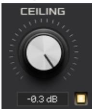
After the Out Gain knob in the signal chain, the Ceiling (when enabled) applies a final stage of 100% hard clipping at the session sample rate with no oversampling, in order to catch any level overages that occur.
