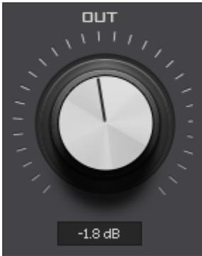
Adjusts the output gain of KClip's oversampled clipper process.
