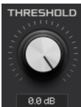
Adjusts the threshold to begin clipping at, all the way down to -48dB. Allows you to clip extremely quiet sources without changing their input gain.
